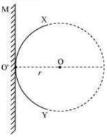
A circle is drawn from the centre (O) such that it just touches the plane mirror at point O'. According to Huygens' Principle, XY is the wavefront of incident light. If the mirror is absent, then a similar wavefront X'Y' (as XY) would form behind O' at
