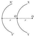
X'Y' can be considered as a virtual reflected ray for the plane mirror. Hence, a point object placed in front of the plane mirror produces a virtual image whose distance from the mirror is equal to the object distance (*r*).
