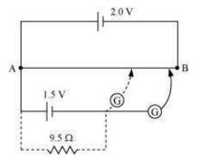
Answer Internal resistance of the cell = rBalance point of the cell in open circuit,  $I_1$  = 76.3 cm
