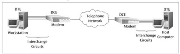
DTE (Data terminal Equipment) : It connects computers to a WAN with the help of a DCE . DTE is end –user equipment , such as a router or computer =  $3919.2 \times 1000 = 3919200$
